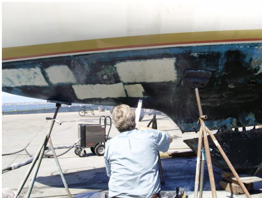
Figure 4-5. Stripping Tests at Marine Group
