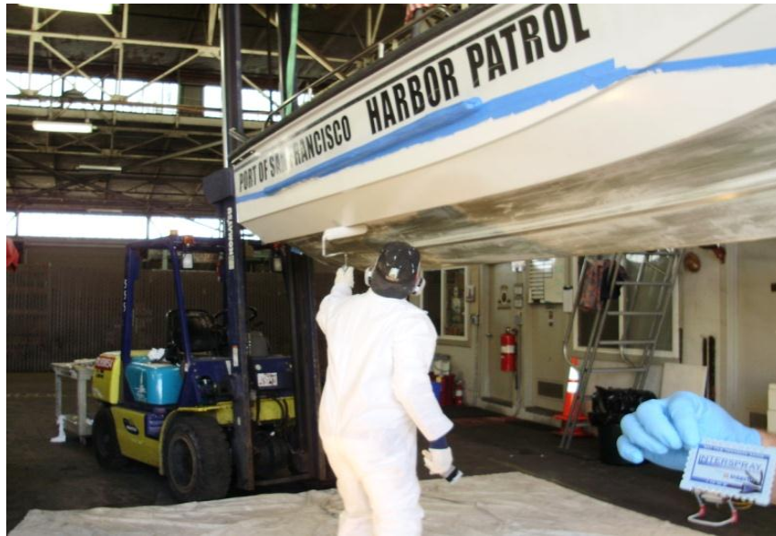
Figure 4-8. Painter Rolling Paint on Boat.
