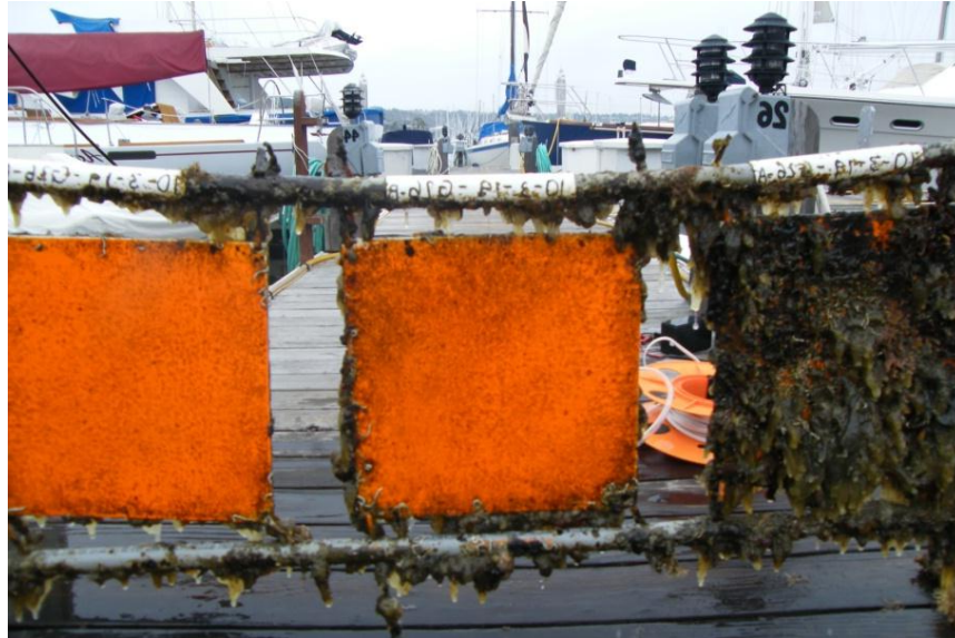
Figure 3-11. Crystal Marine Pro Paint During Panel Testing
