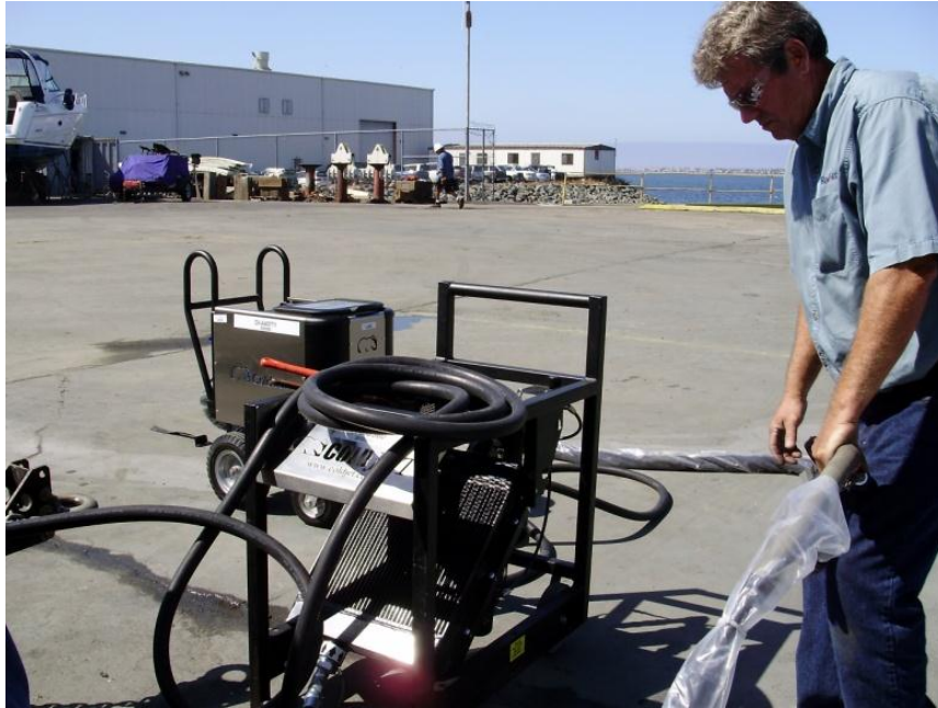
Figure 4-3. Dry Ice Blasting System
