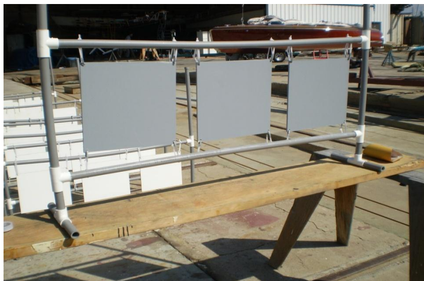
Figure 3-1. Typical Panel Frame
