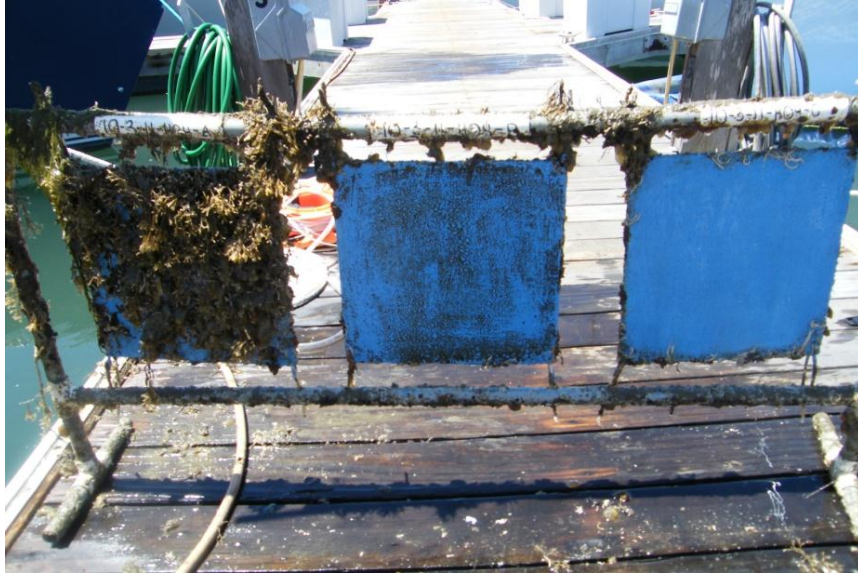
Figure 3-10. HullSpeed 3080 Paint During Panel Testing
