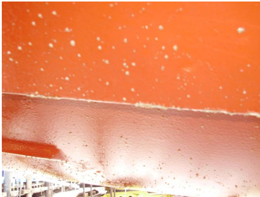
Figure 5-7. Small Barnacles on Port of San Francisco Boat Hull
