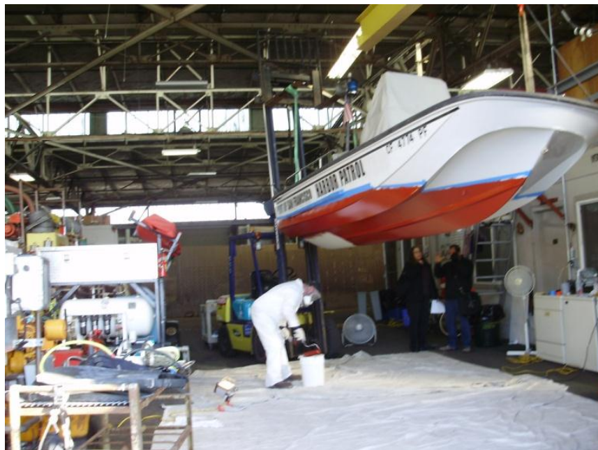
Figure 5-5. Painter Applying Topcoat.
