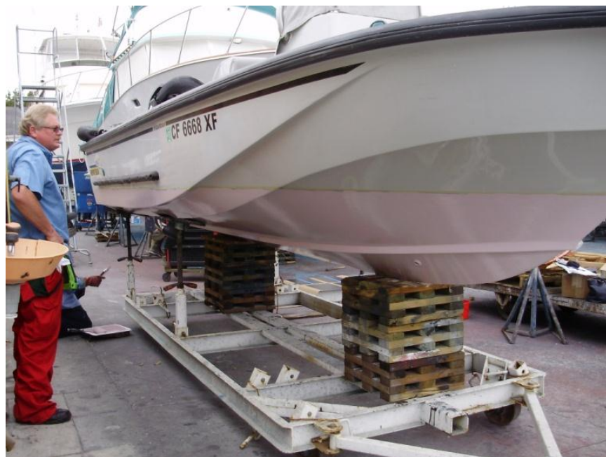
Figure 5-13. City of Newport Beach Boat After Tiecoat Application
