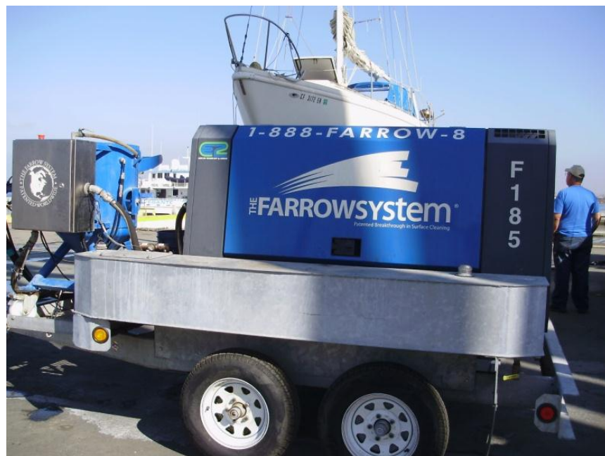
Figure 4-2. Volcanic Rock Blasting System
