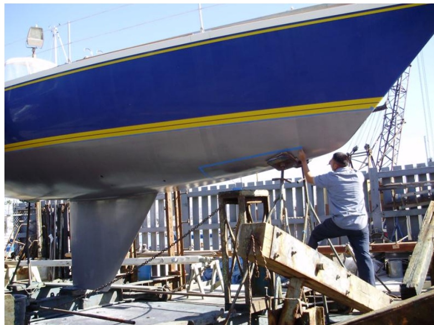
Figure 5-31. Painter Applying Intersleek 900 Topcoat
