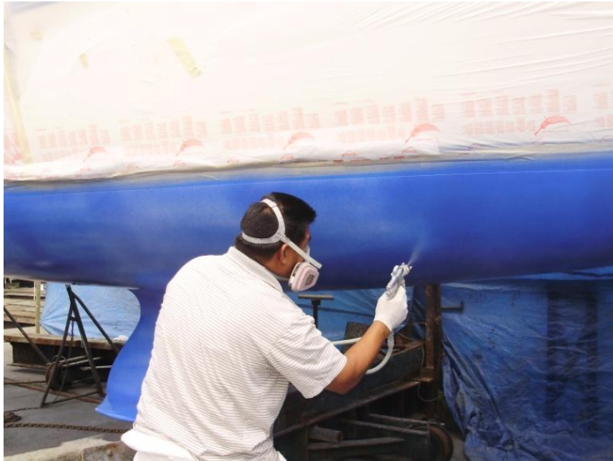
Figure 5-1. Painter Spraying Paint on Auerbach Boat
