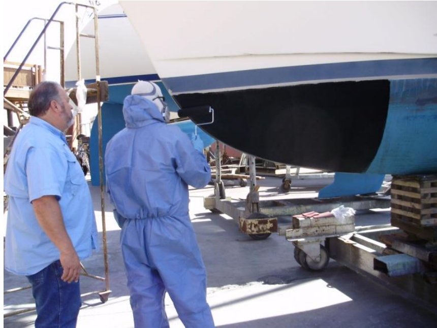
Figure 5-18. Painter Applying Paint to Heinem Boat
