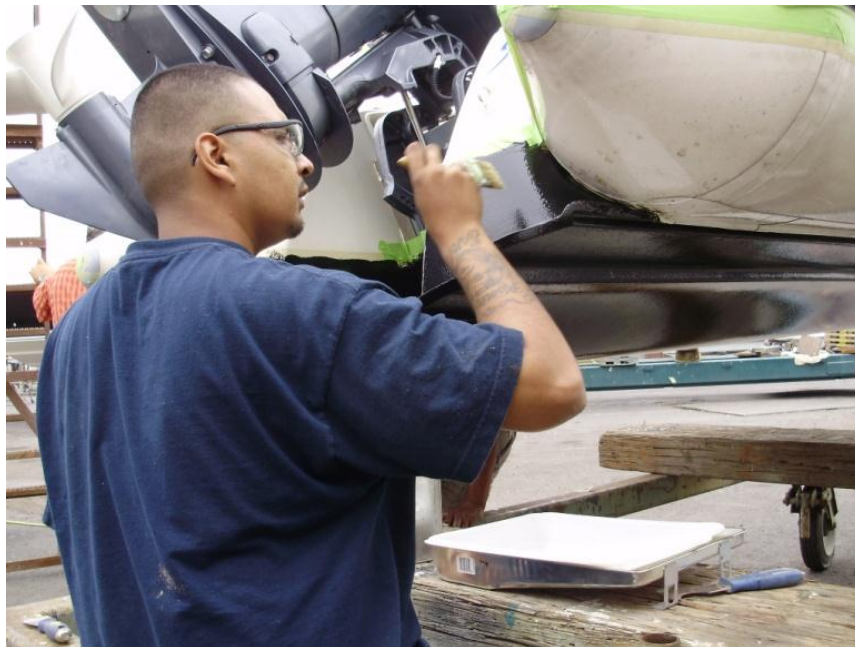
Figure 5-22 Painter Applying Paint to Back of Pasha Boat
