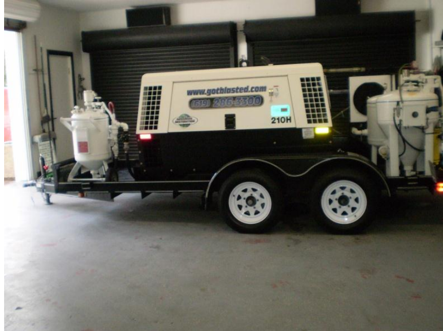
Figure 4-1. Sodium Bicarbonate Stripping System
