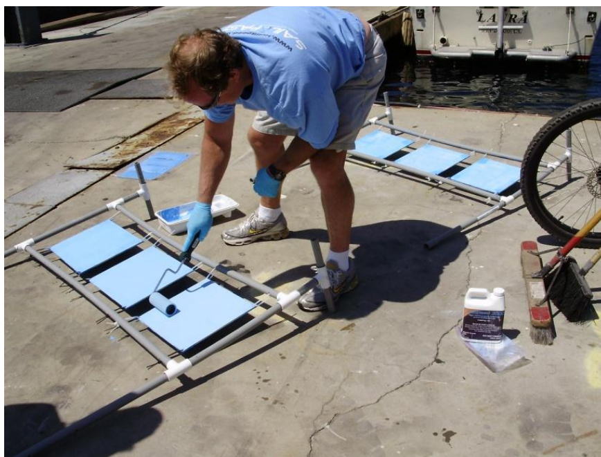
Figure 3-2. Supplier Rolling Paint on Panels
