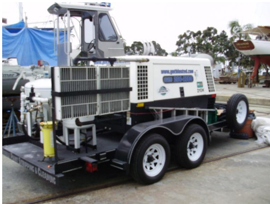
Figure 5-27. Sodium Bicarbonate Stripping System at Boatyard
