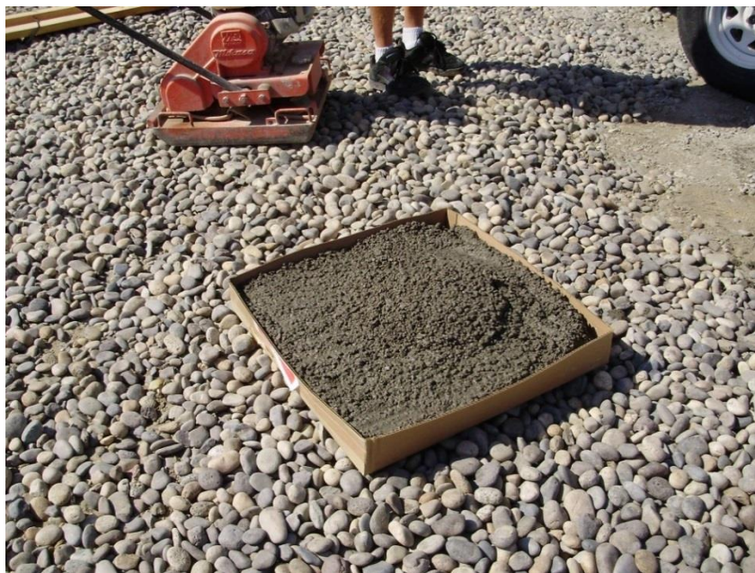
Figure 2-7 Poured Concrete for Dodge Oil Release Agent Field Test
