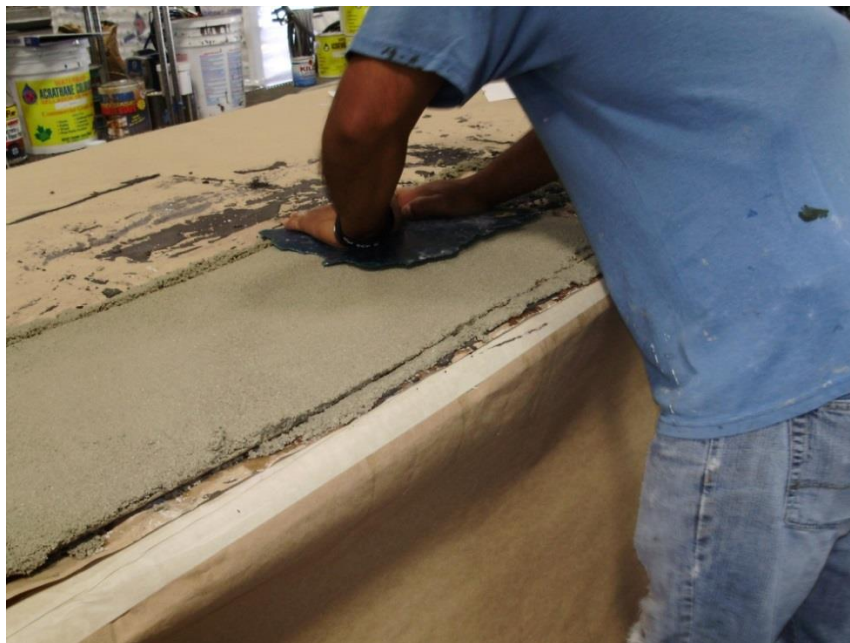
Figure 2-11 Testing Fluoropolymer Coating on Stamp Mat
