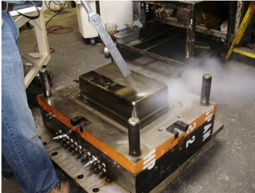
Figure 3-18 Testing Dry Ice Blasting System on Metal Mold
