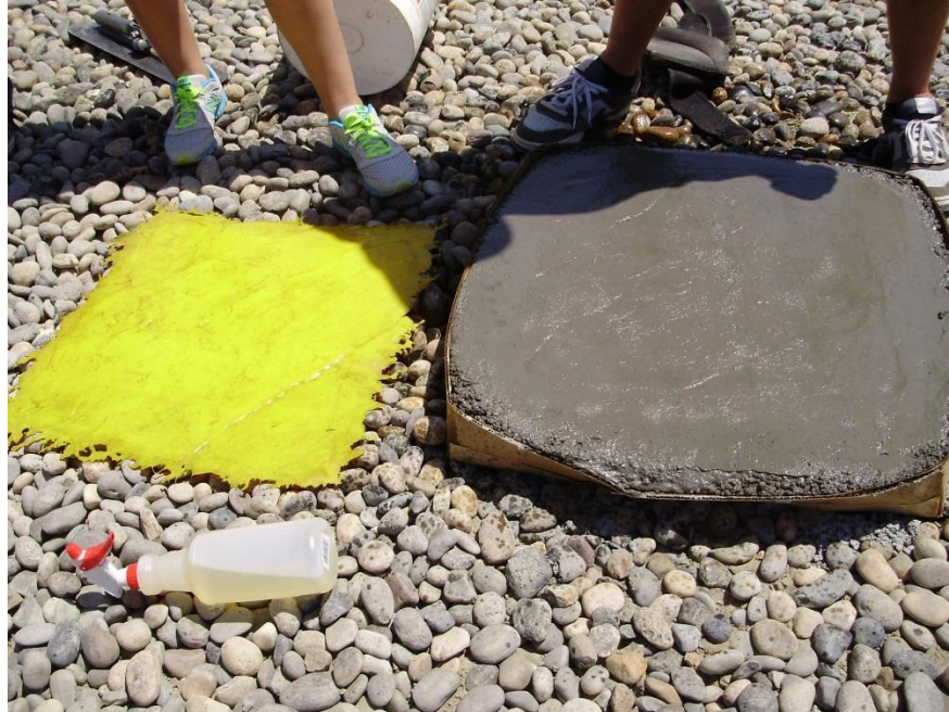
Figure 2-8 Stamp Mat and Concrete After Stamping for Dodge Oil Release Agent
