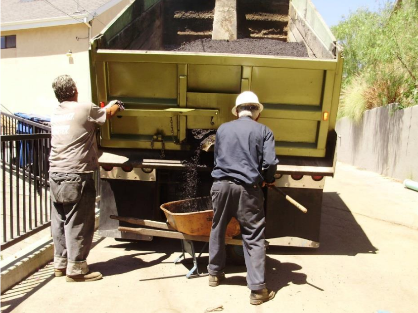
Figure 2-23 Release Agent Testing on Truck Liftgate
