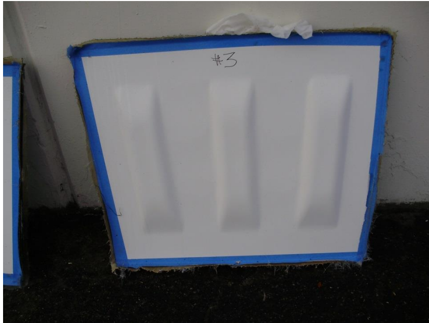
Figure 3-3 Part Made with Water-Based Mold Release Agent
