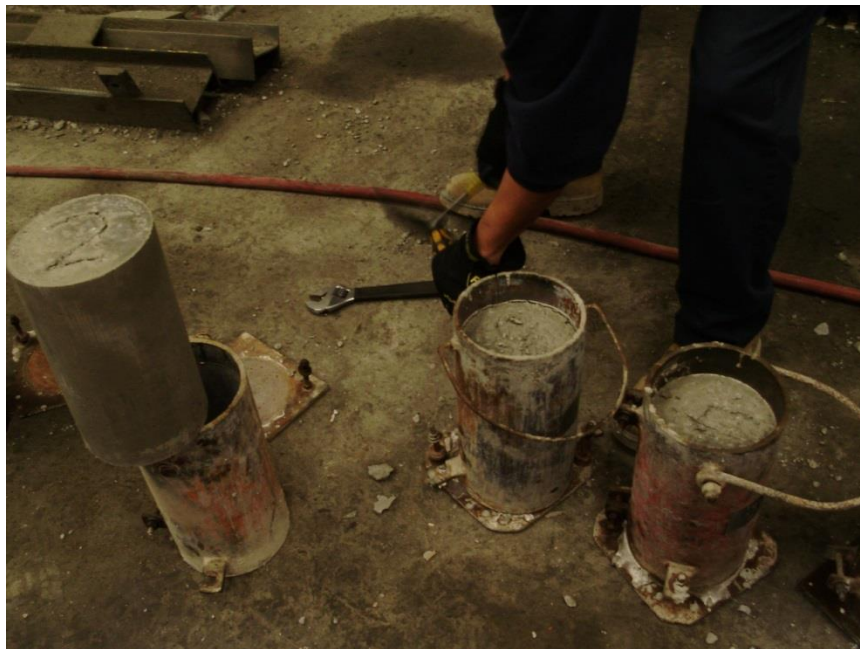
Figure 3-14 Removing Concrete from Testing Devices at Oldcastle Precast
