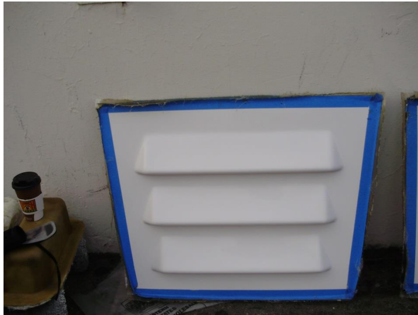
Figure 3-4 Part Made with PTBCF Mold Release Agent
