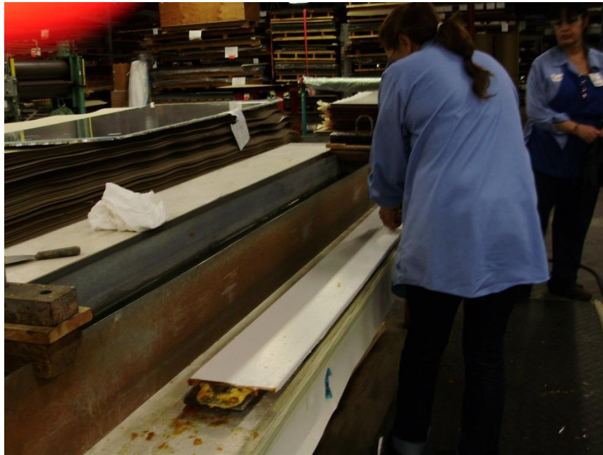
Figure 3-11 Water Bath at M.C. Gill
