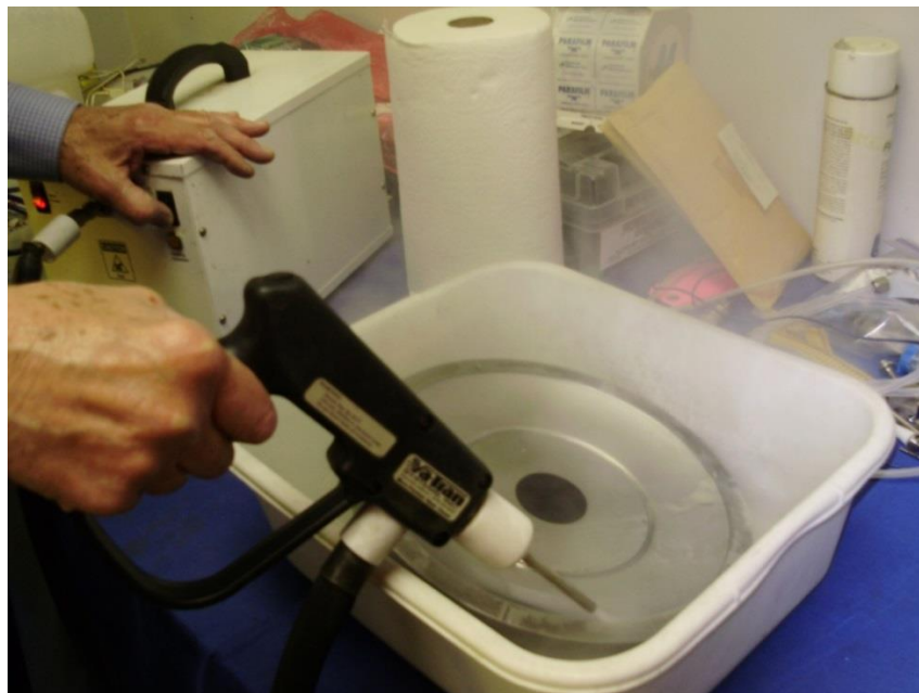
Figure 3-17 Testing Alternative Cleaner on Metal Mold
