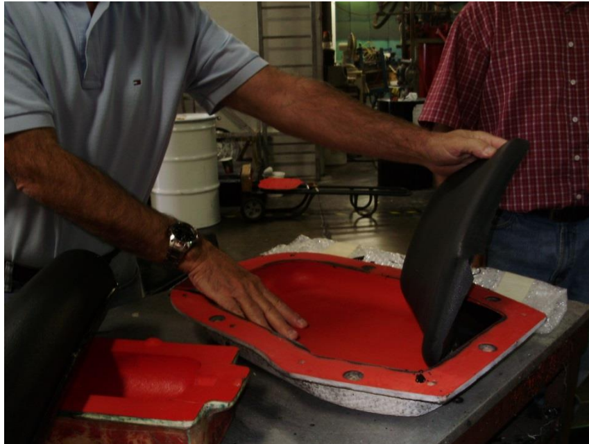
Figure 3-8 Flat Part Made with Mold Release Agent at Fold Molders
