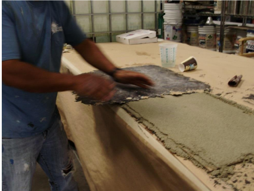
Figure 2-12 Testing Silicone Coating on Stamp Mat
