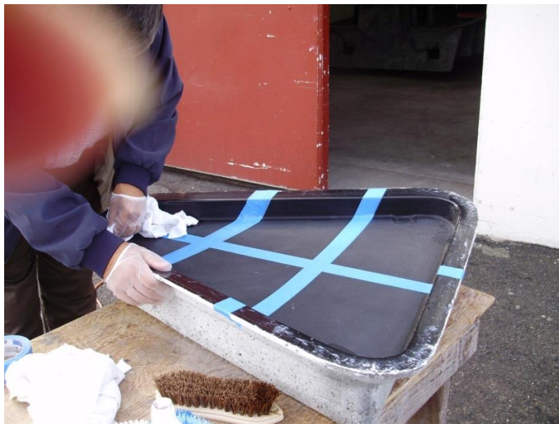
Figure 3-2 Cleaning Test of PCBTF at Boat Manufacturer
