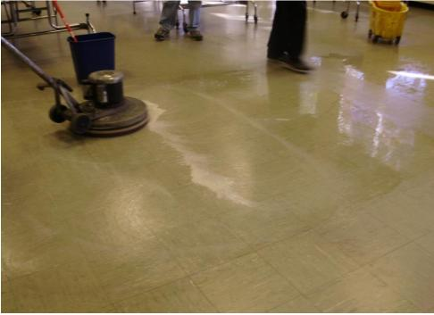
Figure 2-2. Floor Machine Stripping Wax
