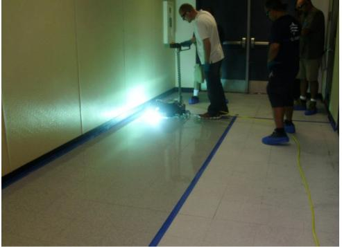
Figure 3-9. Floor Machine with UV Lights
