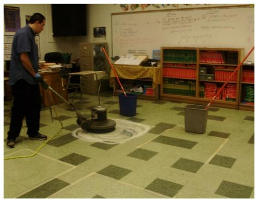
Figure 2-6. Hi-Pro Pad on Floor Machine during Tests at Riverside USD
