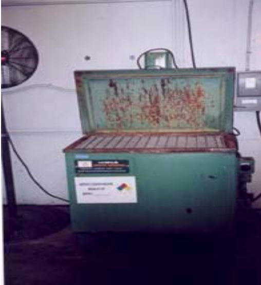
Figure 2-8. Agilift Cleaning System at Multichrome
