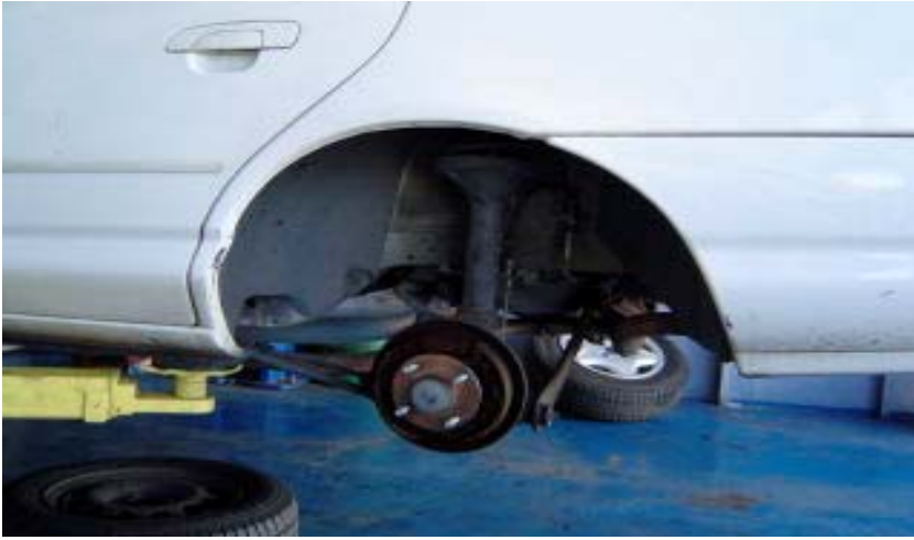
Figure 4-6. Vehicle With Brakes Exposed
