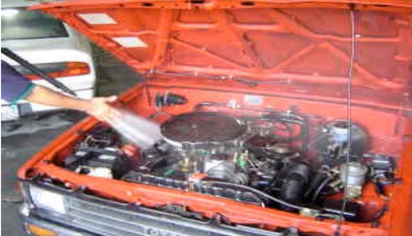
Figure 4-1. Detailer Applying Water-Based Cleaner to Engine
