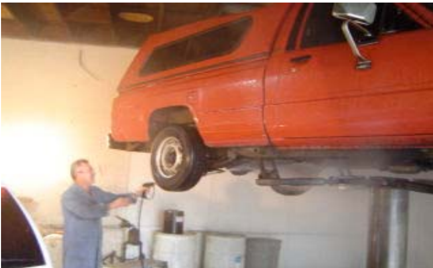
Figure 4-3. Detailer Cleaning Undercarriage of Truck
