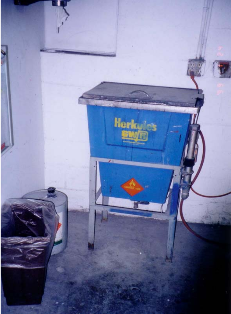
Figure 3-4. Spray Gun Cleaning System at Westway.
