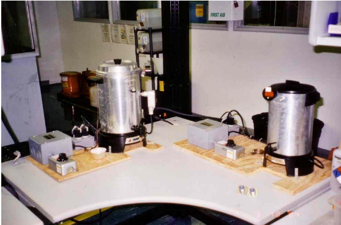
Figure 2-2. Connector Coffee Pot Cleaning System at Hydro-Aire
