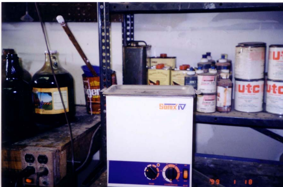
Figure 3-2. Tabletop Ultrasonic Cleaning Unit at Bausman & Father.
