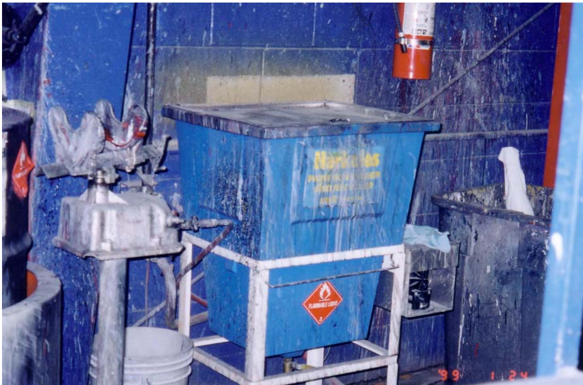
Figure 3-3. Spray Gun Cleaning System at Holmes.
