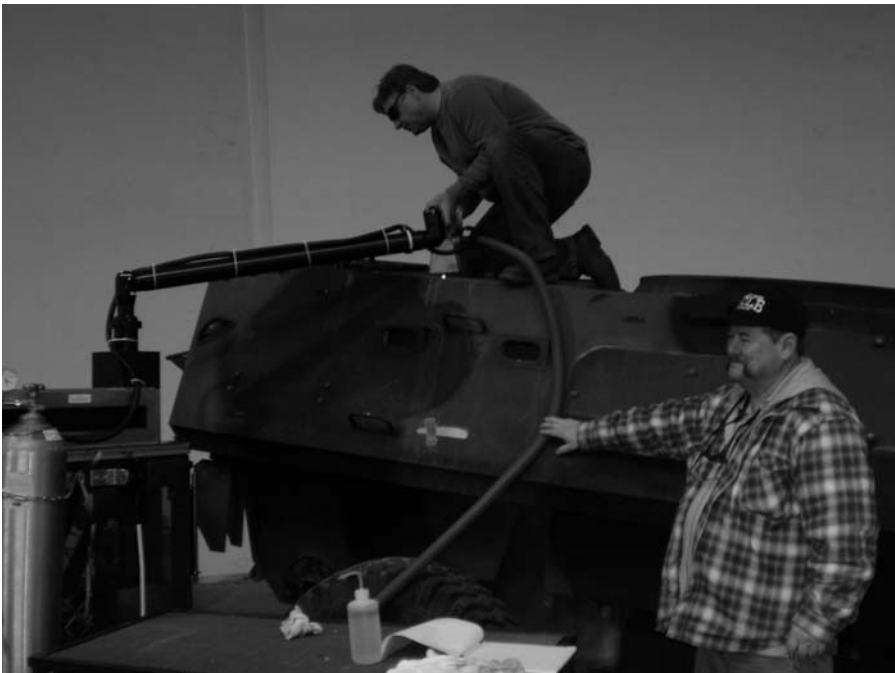
Light Armored Vehicle (LAV) Being Stripped with Laser
