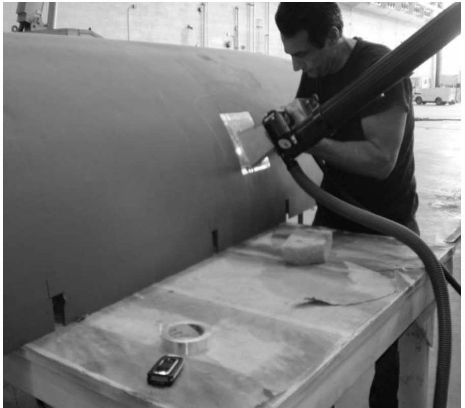
Engine Cowling Being Stripped with Laser
