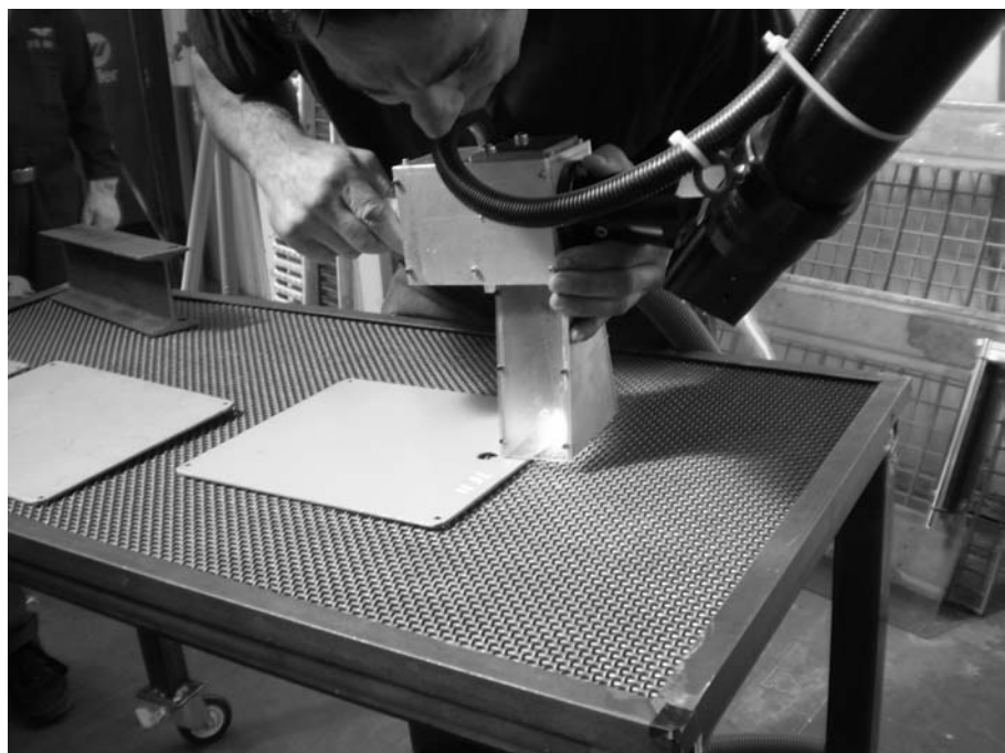
Navy Panels Containing Antifouling Coatings Being Stripped with Laser
