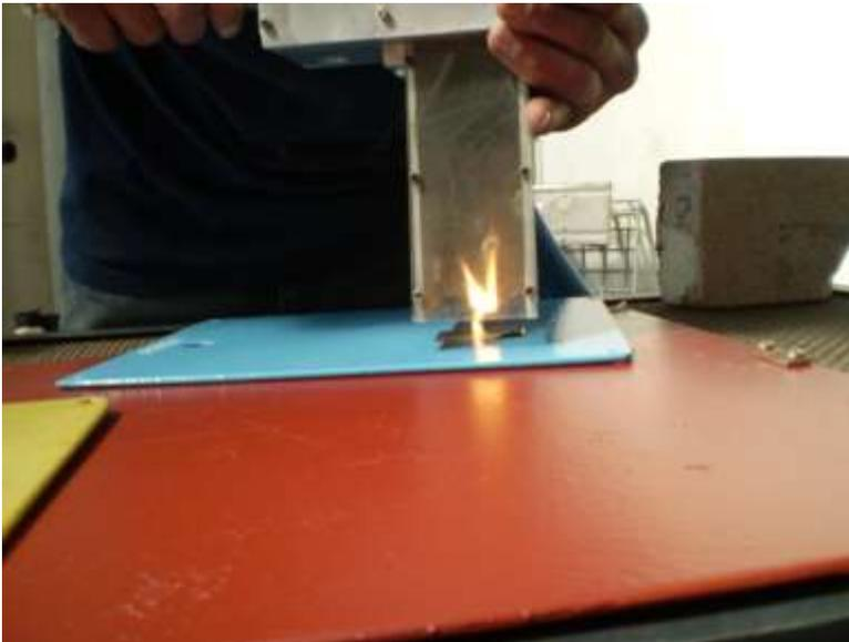
Figure 5-7. Laser Stripping Blue Coated Panel
