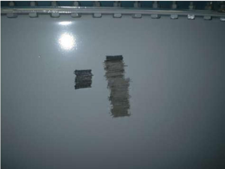
Figure 3-8. Sections Stripped by Laser
