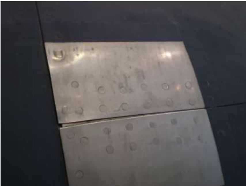
Figure 2-6. Cowling after Stripping
