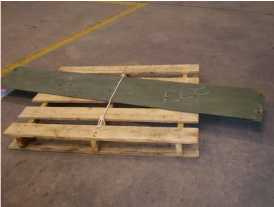
Figure 4-6. Front Plate for Armored Humvee
