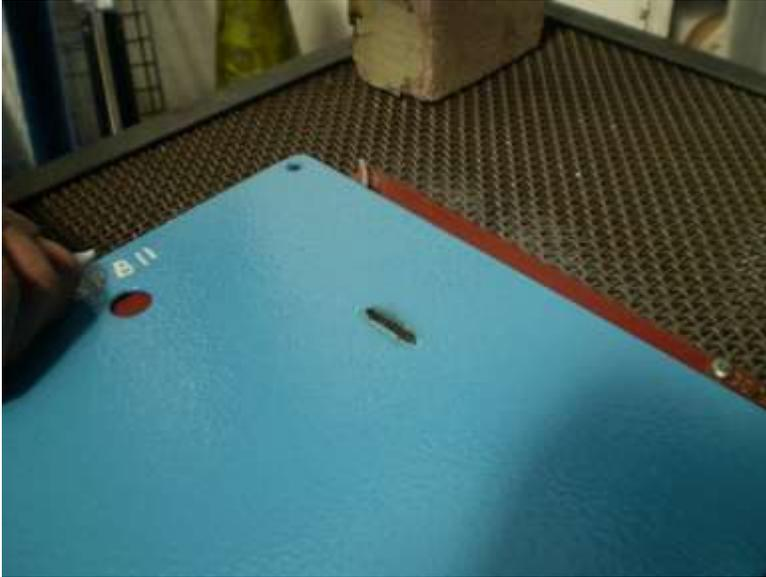
Figure 5-8. Blue Coated Panel after Stripping
