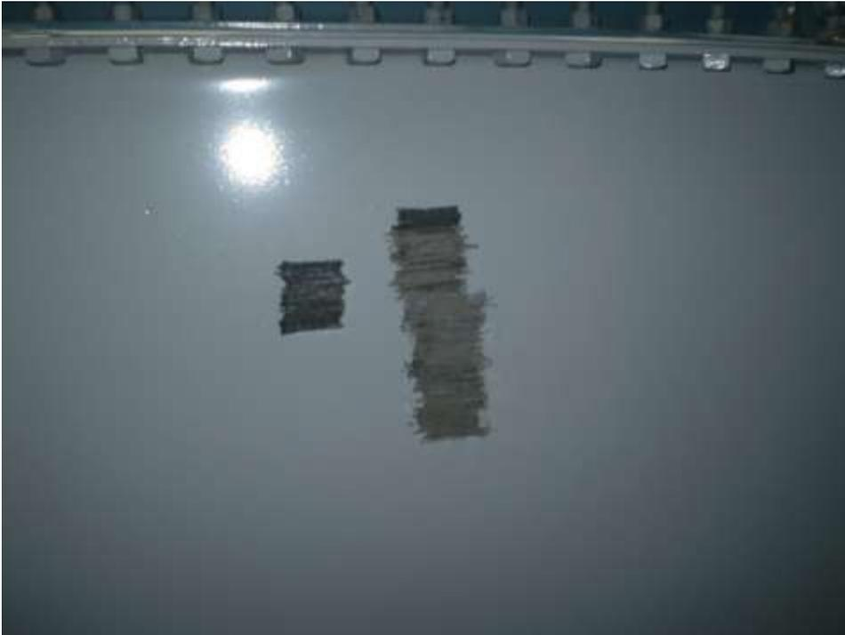
Figure 3-8. Sections Stripped by Laser
