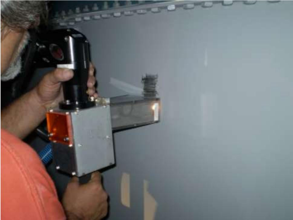
Figure 3-7. Laser Stripping Coating
