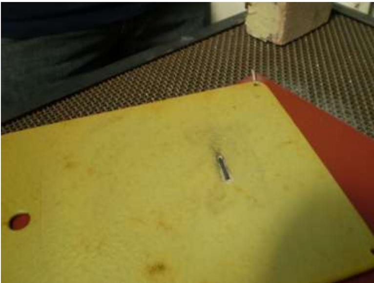
Figure 5-9. Yellow Coated Panel after Stripping
