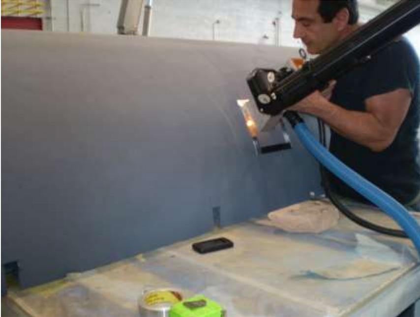
Figure 2-5. Cowling Being Stripped
