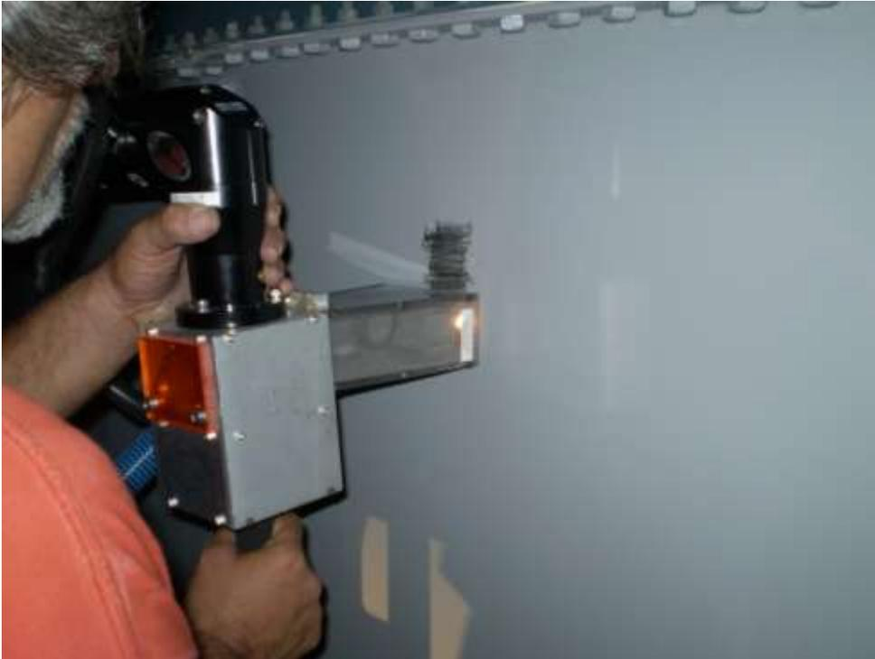
Figure 3-7. Laser Stripping Coating
