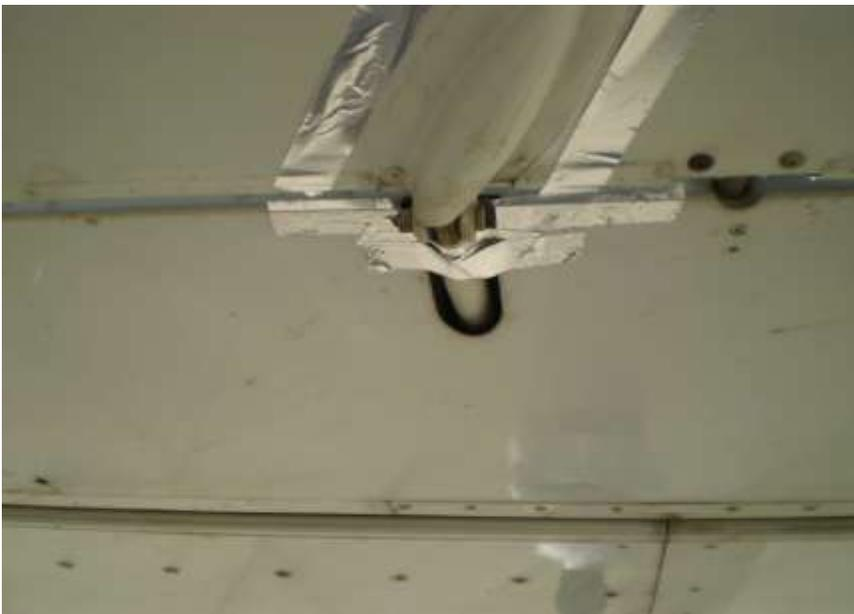
Figure 2-10. Aileron Taped Off
