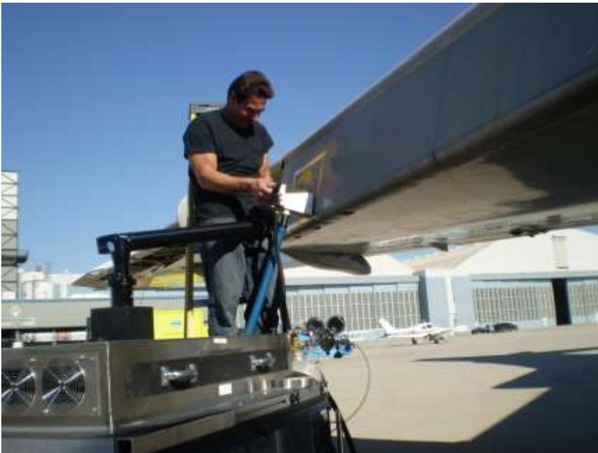
Figure 2-8. Krueger Flap Being Stripped
