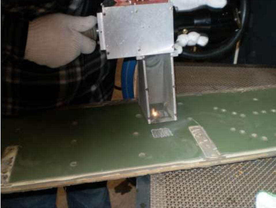
Figure 4-7. Stripping Humvee Front Plate
