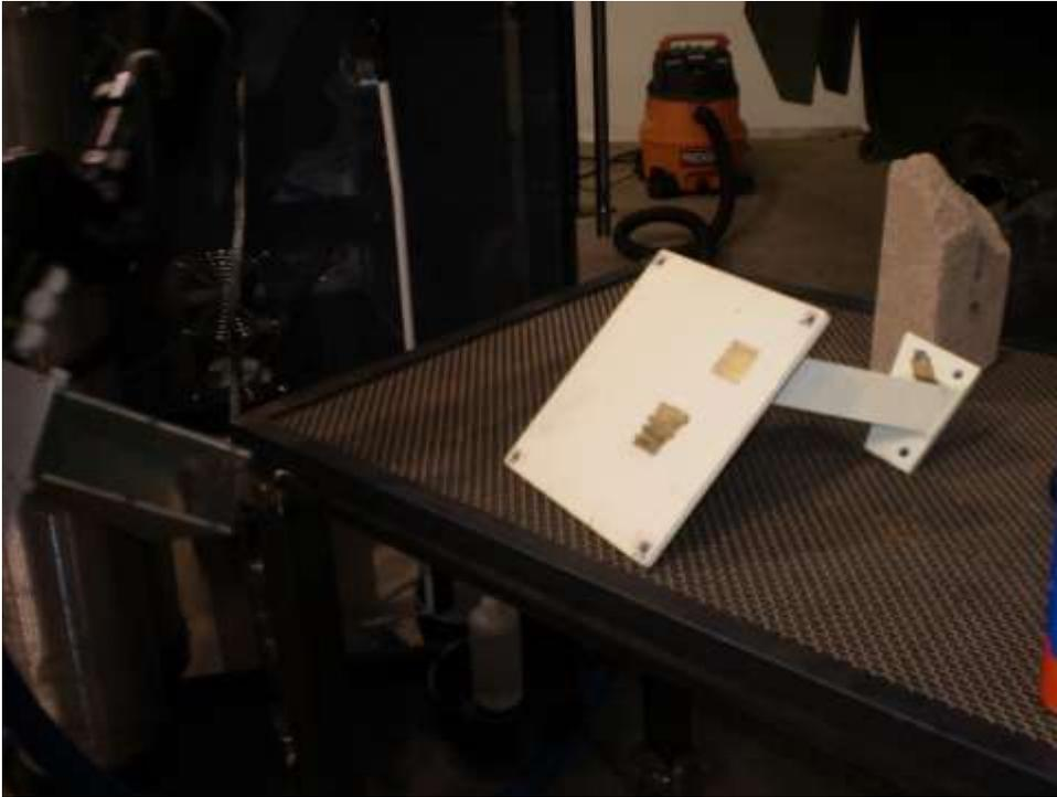
Figure 4-15. Anodized Aluminum Part after Stripping
