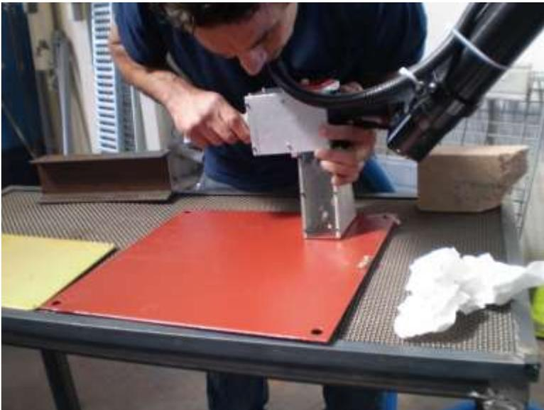
Figure 5-5. Laser Stripping Copper Paint Panel
