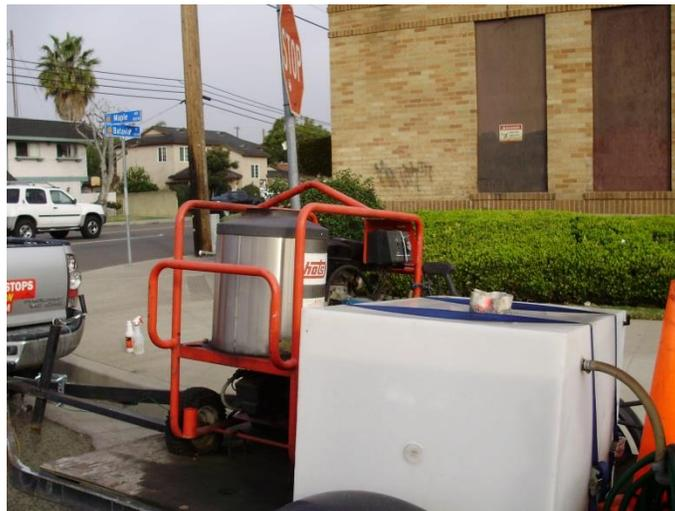
Figure 2-5. Soda blasting system
