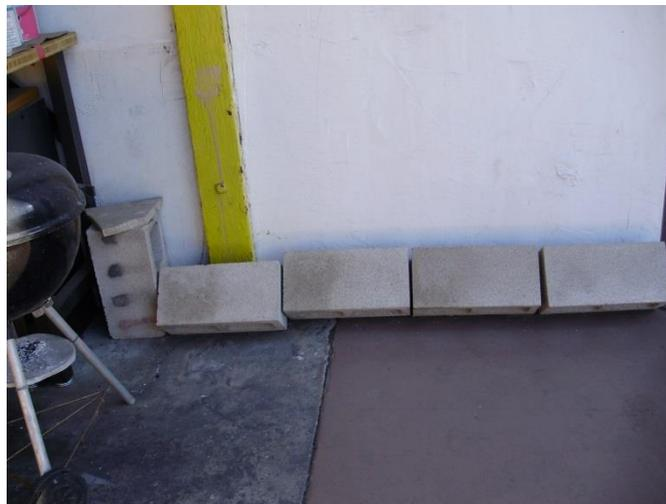
Figure 6-7. Residue remaining on concrete blocks
