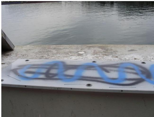
Figure 5-14. Coval coating on fiberglass panel with graffiti
